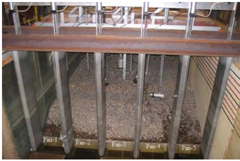
Figure 1. Weighing pans located at the downstream end of the experimental Main Channel.
