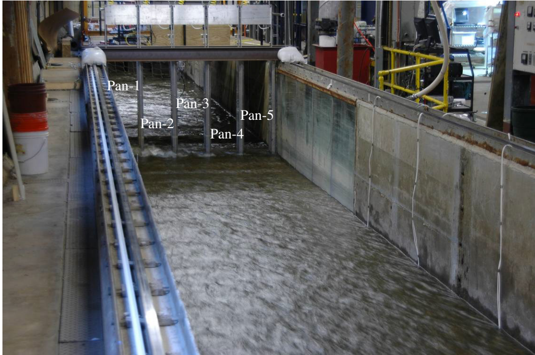
Figure 2. Weighing Pans located at the downstream end of the test channel. The experiment was conducted at the St. Anthony Falls Laboratory, National Center for Earth-surface Dynamics, University of Minnesota.
