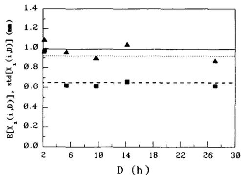
Fig. 11. Stationary models: empirical and theoretical mean (squares and long-dashed line) and standard deviation (triangles and short-dashed line for model 1, solid line for model 2, respectively) of hourly rainfall depths as a function of duration.
