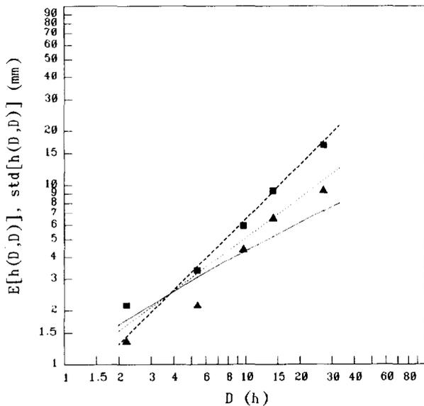
Fig. 8. Stationary models: empirical and theoretical means (squares and long-dashed line, respectively) and standard deviations (triangles and short-dashed line for model 1, solid line for model 2, respectively) of total storm depths as a function of storm duration (log-log plot).
