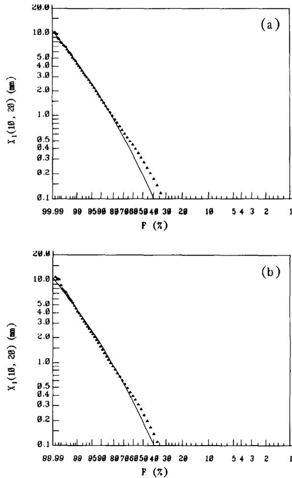
Fig. 13. Theoretical (solid line) and simulated (triangles) distribution function of the incremental depth  $X_1(10, 20)$  (the tenth-hourly depth of a storm with duration 20 hours). The simulated distribution is obtained (a) by the sequential model and (b) by the disaggregation model.
