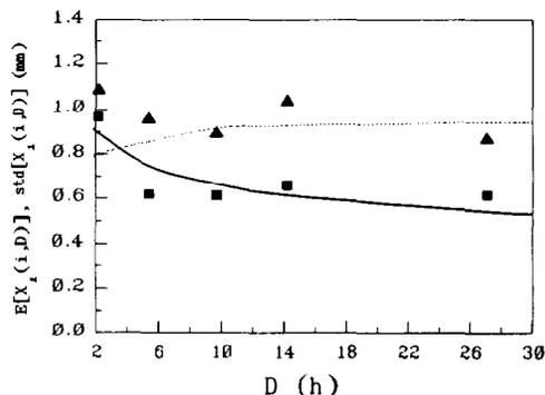
Fig. 6. Scaling model: empirical and theoretical mean (squares and solid line, respectively) and standard deviation (triangles and dashed line, respectively) of hourly rainfall depths as a function of duration.
