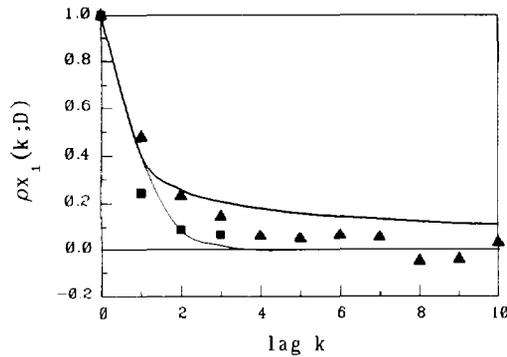
Fig. 12. Stationary models: empirical and theoretical autocorrelation function of hourly rainfall depths as a function of duration. Squares and triangles represent empirical values for small ( $4 \text{ hours} \leq D \leq 11 \text{ hours}$ ) and large durations ( $12 \text{ hours} \leq D \leq 45 \text{ hours}$ ), respectively, while thick and thin lines represent models 1 and 2, respectively (same for all durations).
