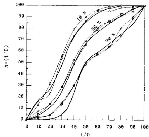
Fig. 15. Comparison of historical and synthetic normalized mass curves of second-quartile storms at Chalara station, province of Macedonia, Greece, for 10%, 50% (median), and 90% probability levels. Synthetic curves (thick solid lines) are obtained from a simulated sample by using the disaggregation procedure. The two groups of historical curves correspond to the records of April (circles) and all months of the year (squares), respectively.
